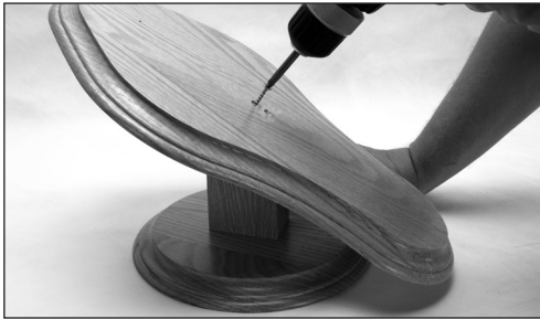
4. Use Template B provided below to predrill two pilot holes in the Brace. (Use the diagram below to see proper placement of the template). Attach the Skull Panel to the other side of the Brace using the 2" screws.
