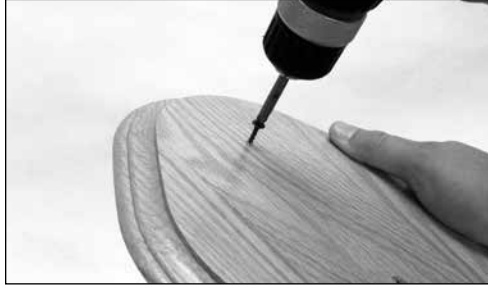
6. Drill a small pilot hole into the location determined in step 5. Screw in the 1" screw leaving an adequate amount exposed to hang your skull.
