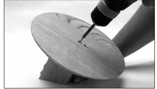
3. Use Template A provided below to predrill two pilot holes in the Base. Attach the Base to the Brace using the 2" screws.
