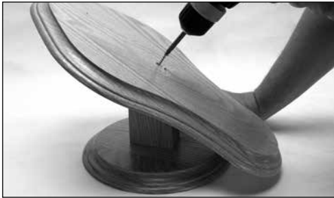
4. Use Template B provided below to predrill two pilot holes in the Brace. (Use the diagram below to see proper placement of the template). Attach the Skull Panel to the other side of the Brace using the 2" screws.
